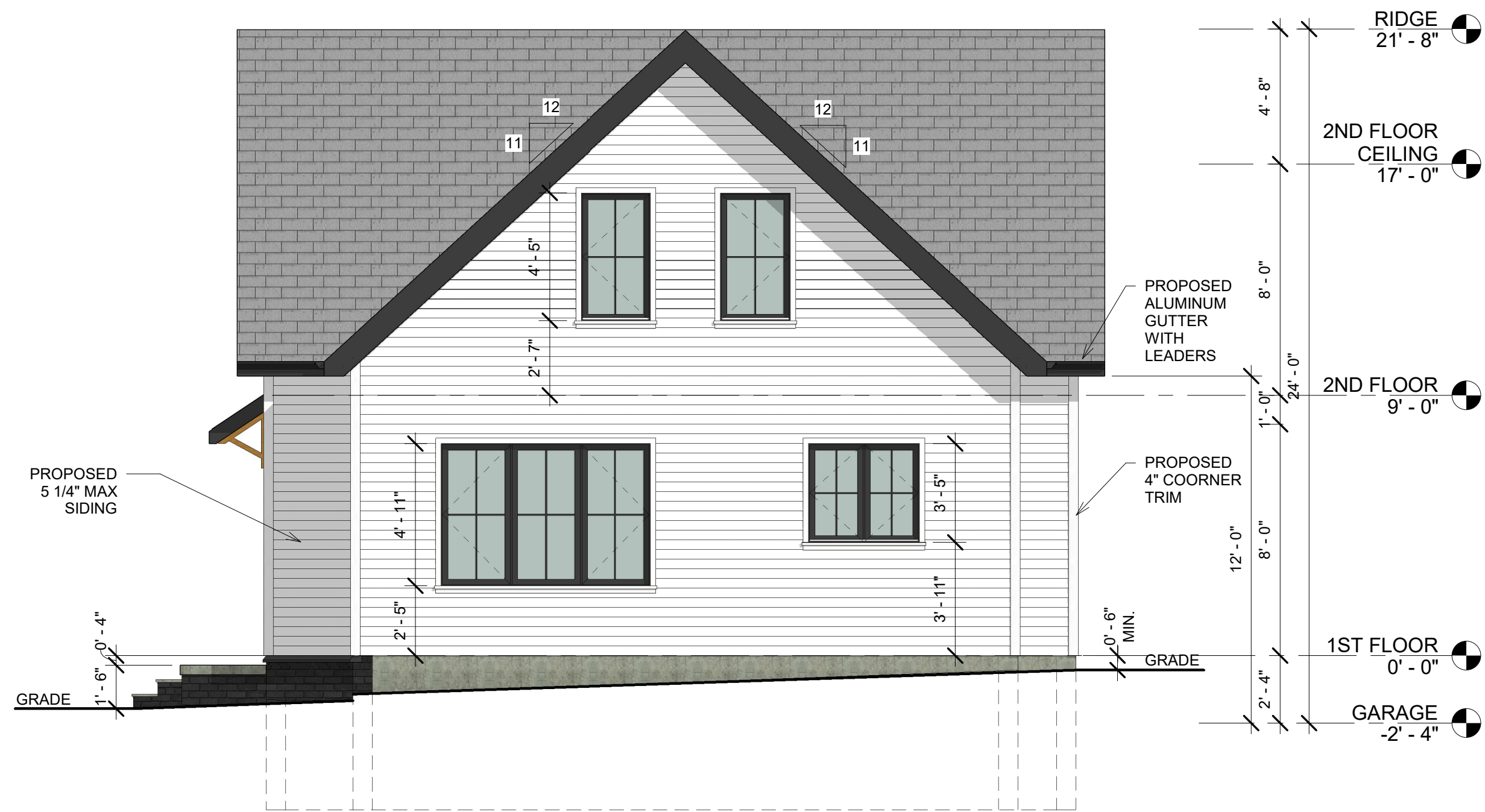
3 PROPOSED RIGHT ELEVATION 1/4" = 1'-0"
