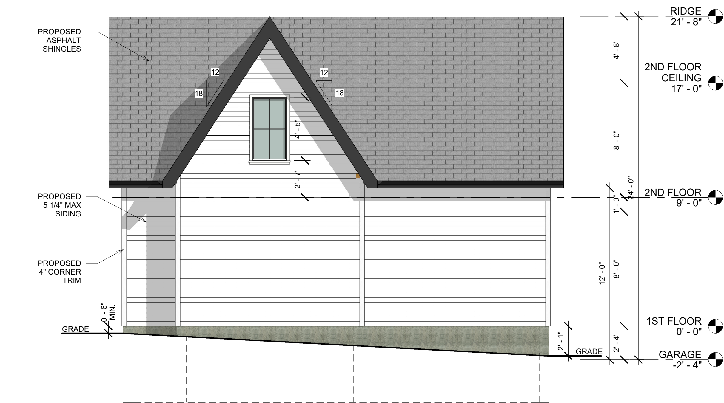
2 PROPOSED REAR ELEVATION 1/4" = 1'-0"
