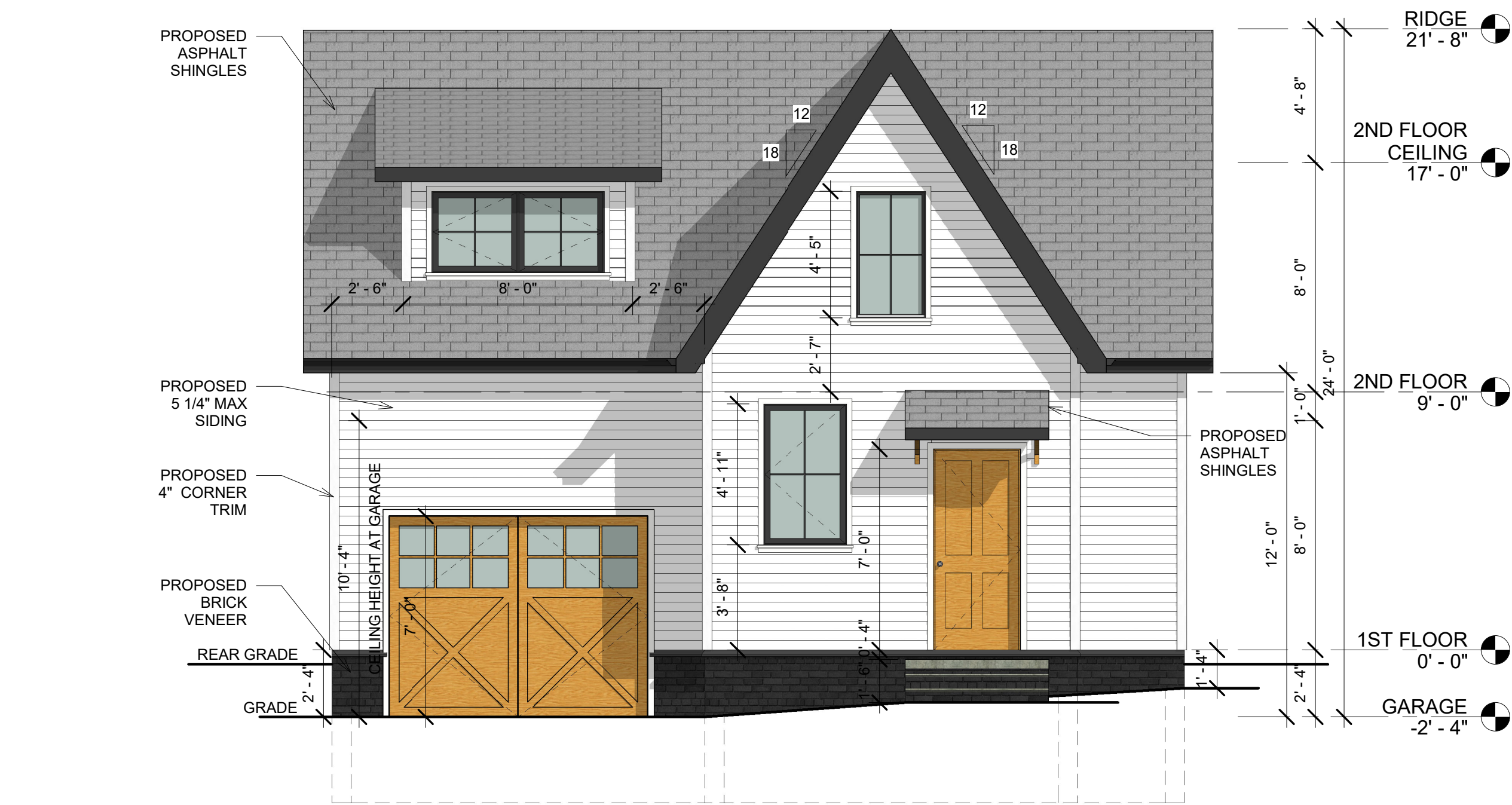
1 PROPOSED FRONT ELEVATION 1/4" = 1'-0"
